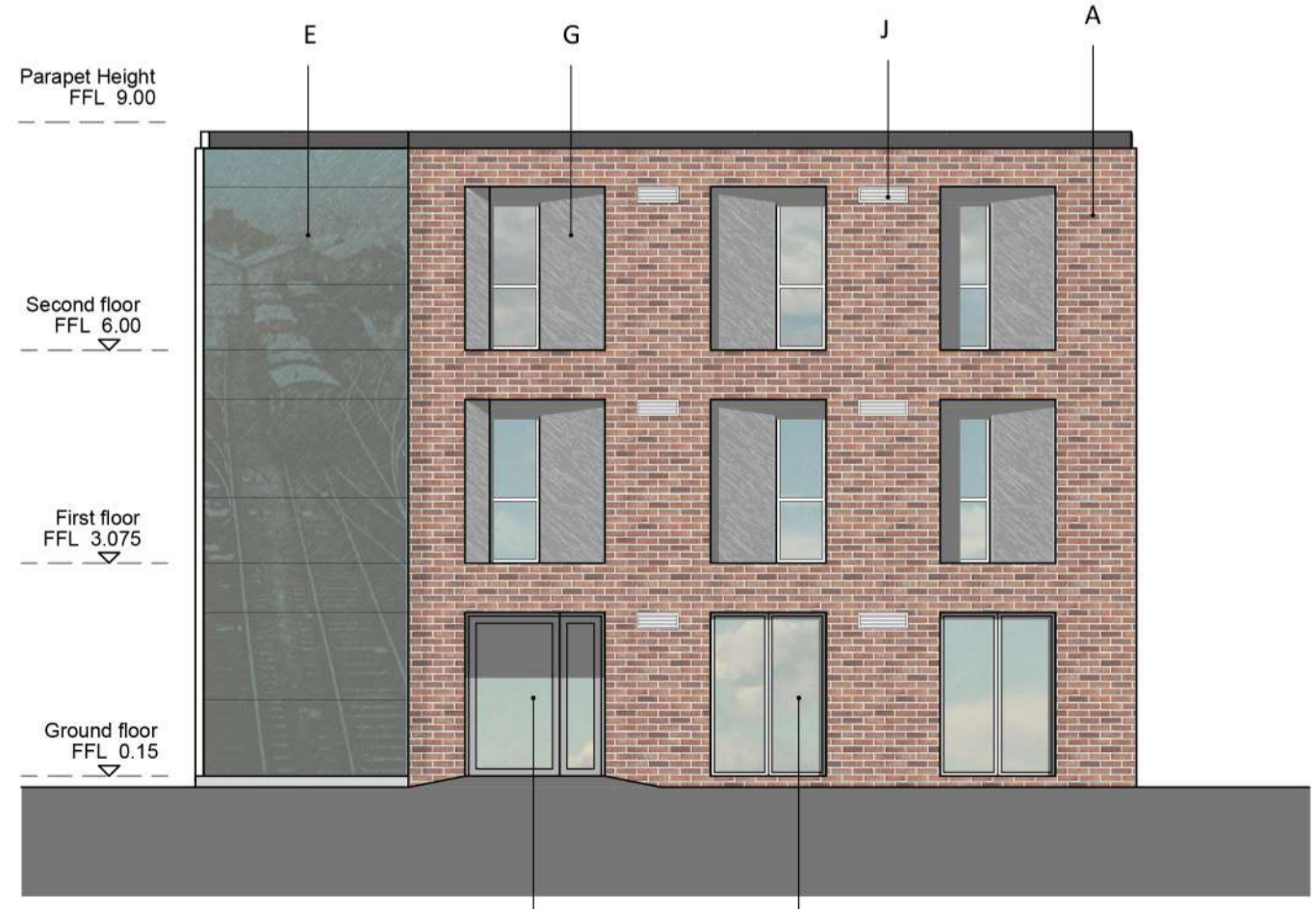
BLOCK C ELEVATION 3 - NORTH-WEST ELEVATION
